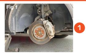
• Before installation, make sure the hub/rotor is securely attached to the vehicle and free of any damage.
